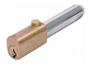
Extruded brass body Body size 14mm x 21mm oval profile, 33mm length Hardened steel bullet, 12.5mm diameter x 45mm length Supplied with 2 numbered keys
